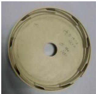
Fig. 2: Flow channel and axial position of diffuser
