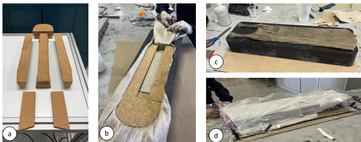
Fig. 4. Prototype manufacturing steps a) Material cutting; b-c) wet lay-up; d) vacuum compaction.
