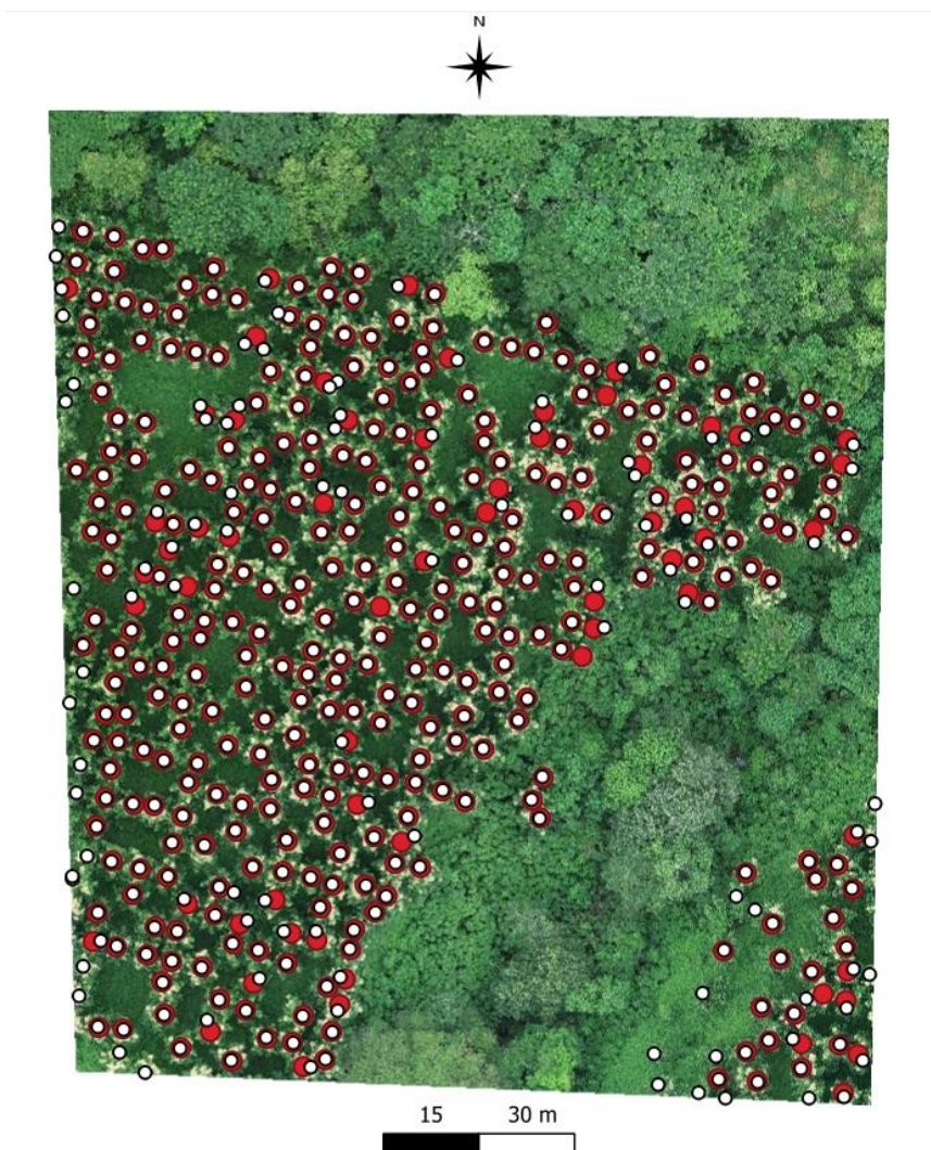
Fig. 5. Test plot number 4 at the “La Selena” teak plantation. The red dots superimposed on the orthoimage represent the geolocation of the teak trees predicted by the YOLOX-small model, while the white dots represent the manually digitized teak trees (ground truth).
