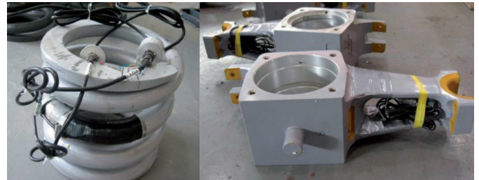
Fig. 4. Measuring Points of Spring and Tumbler Loads
